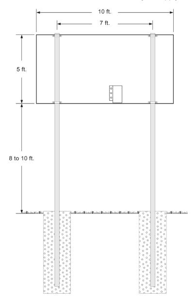
Once you have verified the positions of the posts and the size of the footings, you are ready to dig your holes, pour your concrete, and set your posts. There are several techniques for ensuring proper alignment of the posts. Typically installers will construct a temporary wooden support frame to hold each post in place while the concrete sets. Having plumb posts in the proper position is the key to a smooth mechanical installation.
